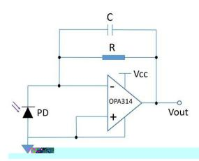
$$V_{out}(V) = I_{ph}(A) \times R(\Omega)$$
